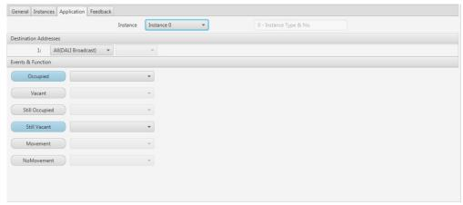
Figure 28-3: Type 303 Occupancy Sensor Instance Application Configuration
