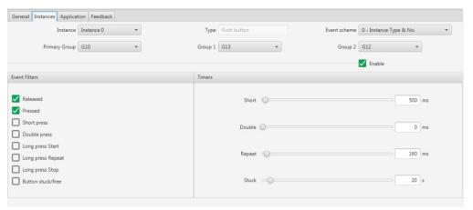
Figure 27-1: Type 301 Push Button Instance Configuration
