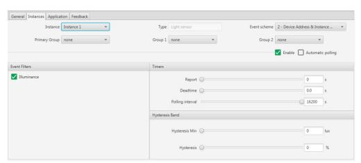
Figure 27-4: Type 304 Light Sensor Input Device Configuration
