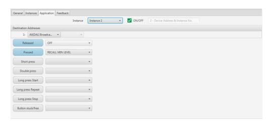
Figure 28-1: Type 301 Push Button Instance Application Configuration
