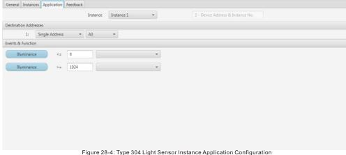
The application configuration of sensor input device instance is to define the upper limitation value and lower limitation value of illuminance, when the actual illuminance value is within the limitation range, the configured command will be triggered.
