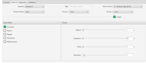
Figure 27-3: Type 303 Occupancy Sensor Input Device Configuration
